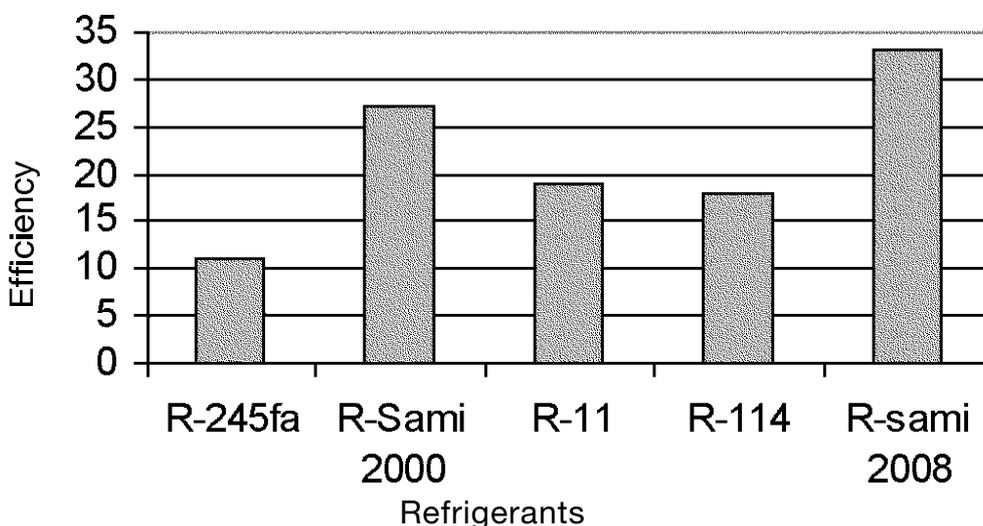
Figure 4 Efficiency for different refrigerants.
